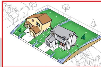
*Split Surface Drainage diagram shows how the swales convey water to the front and back*
