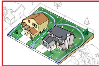
*Rear to Front Surface Drainage diagram shows how the swales direct water away from properties*
